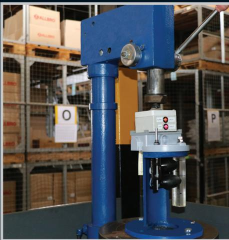
\* Allbro's Buchholz Relay Mechanical & Electrical verification of float and switch functionality
