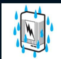
**1** Protected against vertically falling water droplets (condensation)
