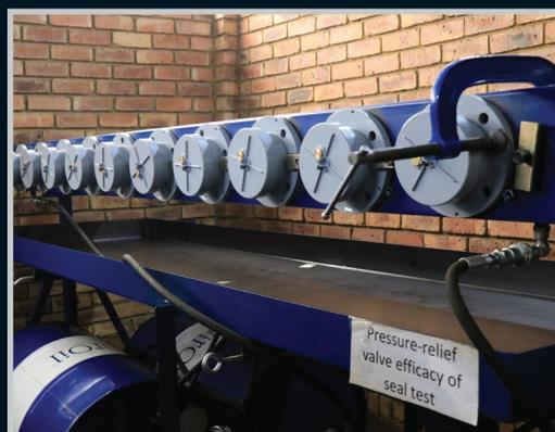
\* Allbro's in-house PRV Efficacy of seal test & Operational Function Test equipment
